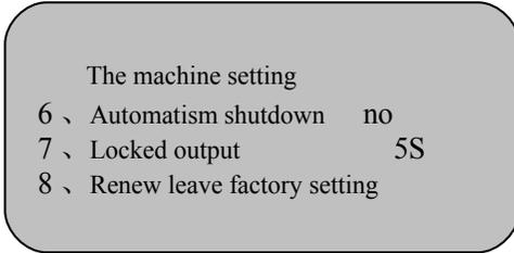
Use OK keys and the arrow keys set parameters, could select close or open, and also set time delay.
